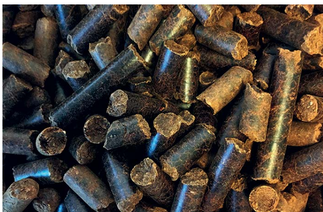
Steam exploded pellets used at Thunder Bay Generating Station (Copyright of photo: Arbaflame AS)
