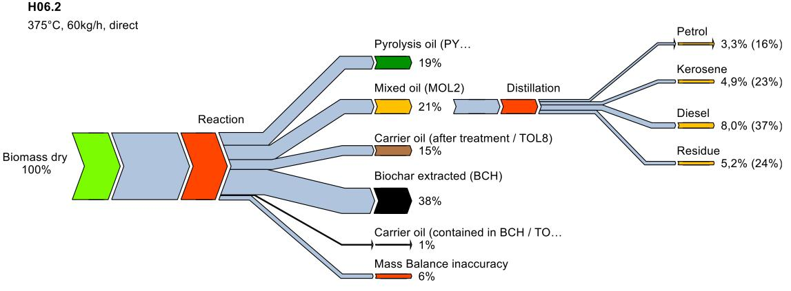
Results from bioCRACK pilot plant Schwechat Feedstock: spruce
